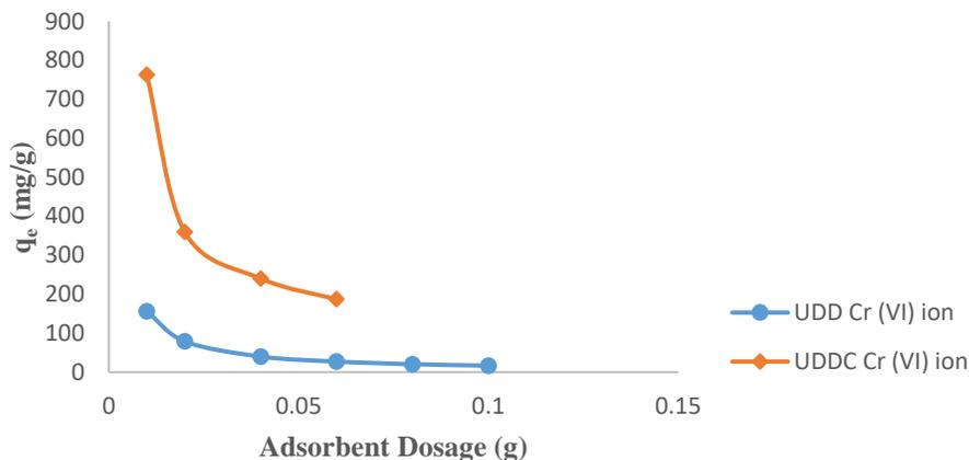
**Figure 4:** Effect of Adsorbent Dosage for Cr (VI) ion onto UDD Peels & UDDC
