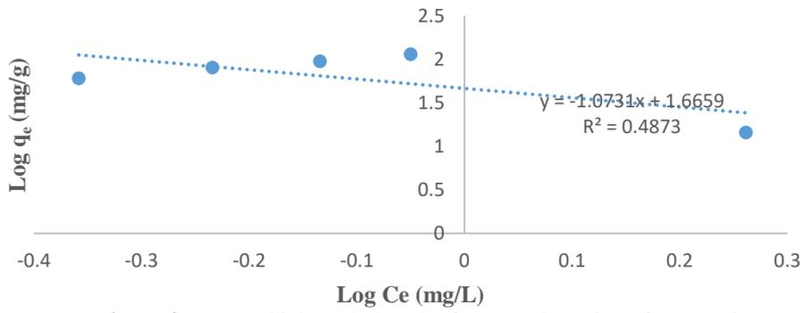
**Figure 9a:** Freundlich Isotherm Plot for the Adsorption of Cr (VI) ion onto UDD peel
