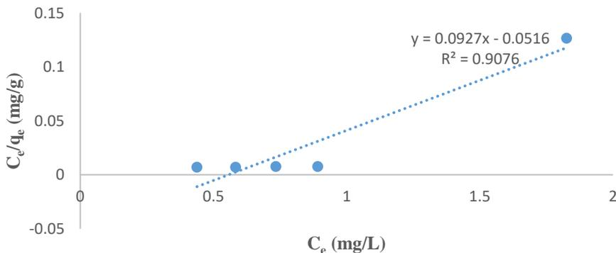
**Figure 8a:** Langmuir Isotherm Plot for the Adsorption of Cr (VI) ion onto UDD
