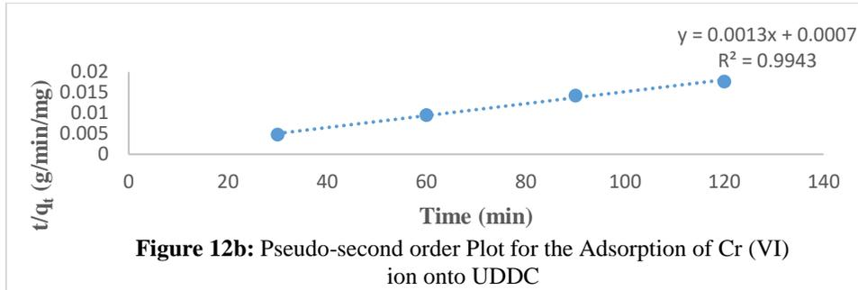
**Figure 12b:** Pseudo-second order Plot for the Adsorption of Cr (VI) ion onto UDDC
