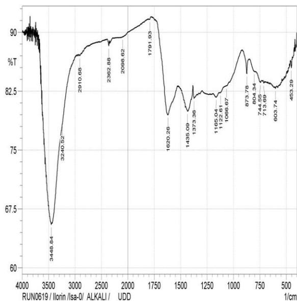
**Figure 2a:** FT-IR spectrum of UDD Peel
