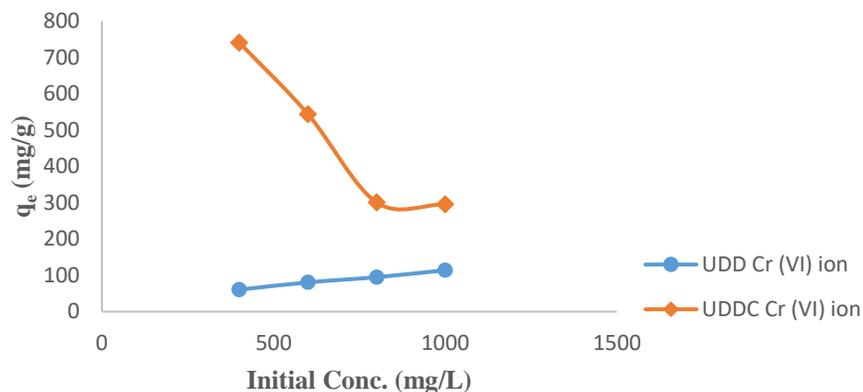
**Figure 3:** Effect of Initial Conc. for Cr (VI) ion onto UDD Peels & UDDC
