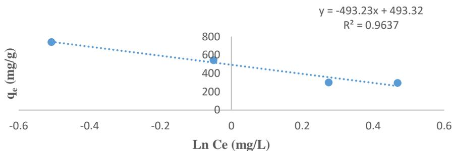
**Figure 10b:** Temkin Isotherm Plot for the Adsorption of Cr (VI) ion onto UDDC
