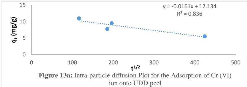
**Figure 13a:** Intra-particle diffusion Plot for the Adsorption of Cr (VI) ion onto UDD peel
