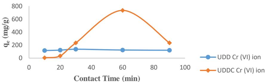
**Figure 5:** Effect of Contact Time for Cr (VI) ion onto UDD Peels & UDDC
