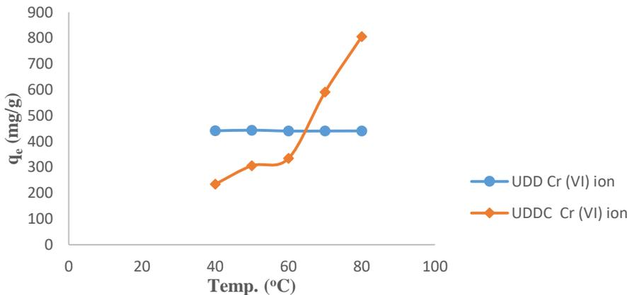
**Figure 7:** Effect of Temp. for Cr (VI) ion onto UDD Peels & UDDC
