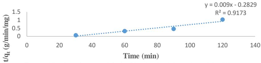
**Figure 12a:** Pseudo-second Order Plot for the Adsorption of Cr (VI) ion onto UDD peel
