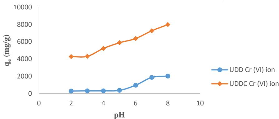
**Figure 6:** Effect of pH for Cr (VI) ion onto UDD Peels & UDDC
