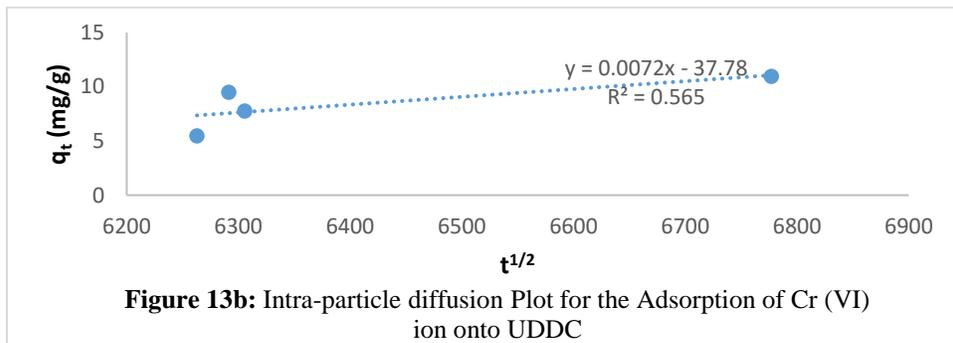
**Figure 13b:** Intra-particle diffusion Plot for the Adsorption of Cr (VI) ion onto UDDC
