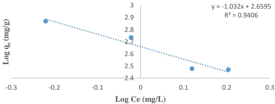
**Figure 9b:** Freundlich Isotherm Plot for the Adsorption of Cr (VI) ion onto UDDC
