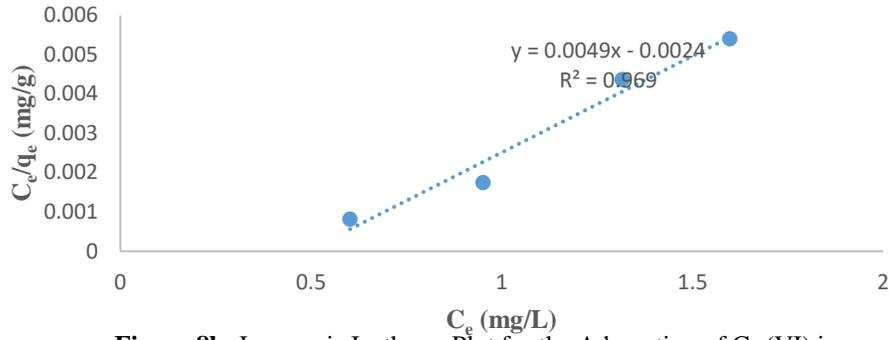
**Figure 8b:** Langmuir Isotherm Plot for the Adsorption of Cr (VI) ion onto UDDC
