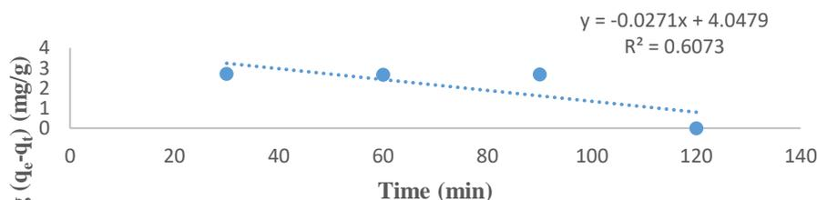
**Figure 11b:** Pseudo-first order Plot for the Adsorption of Cr (VI) ion onto UDDC
