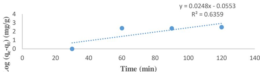
**Figure 11a:** Pseudo-first Order Plot for the Adsorption of Cr (VI) ion onto UDD peel
