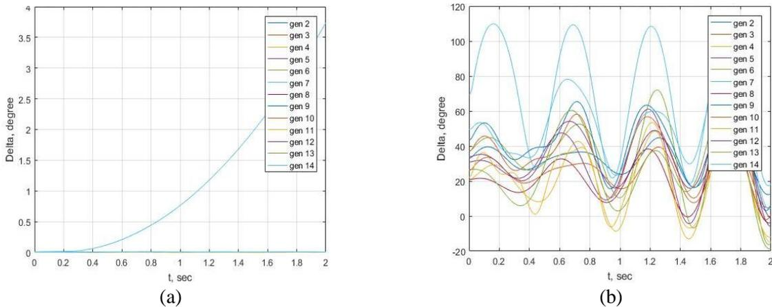
**Figure 8:** Swing curve of three-phase fault on bus 20, line [15-20] of the Nigerian 34-power network and cleared at 0.021 s (a) without STATCOM (b) with STATCOM
