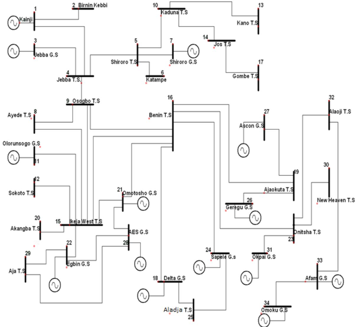
**Figure 2:** Nigerian 14-machine, 34-bus power network (Ikeli, 2019)
