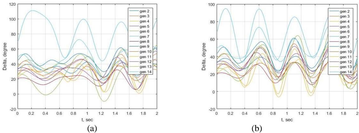
**Figure 6:** Swing curve of three-phase fault on bus 20, line [15-20] of the Nigerian 34-bus power network and cleared at 0.019 s (a) without STATCOM (b) with STATCOM
