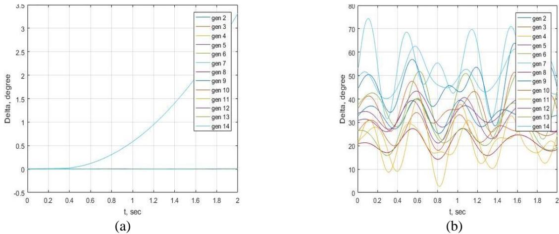
**Figure 11:** Swing curve of three-phase fault on bus 22, line [22-29] of the Nigerian 34-bus power network and cleared at 0.0150 s (a) without STATCOM (b) with STATCOM
