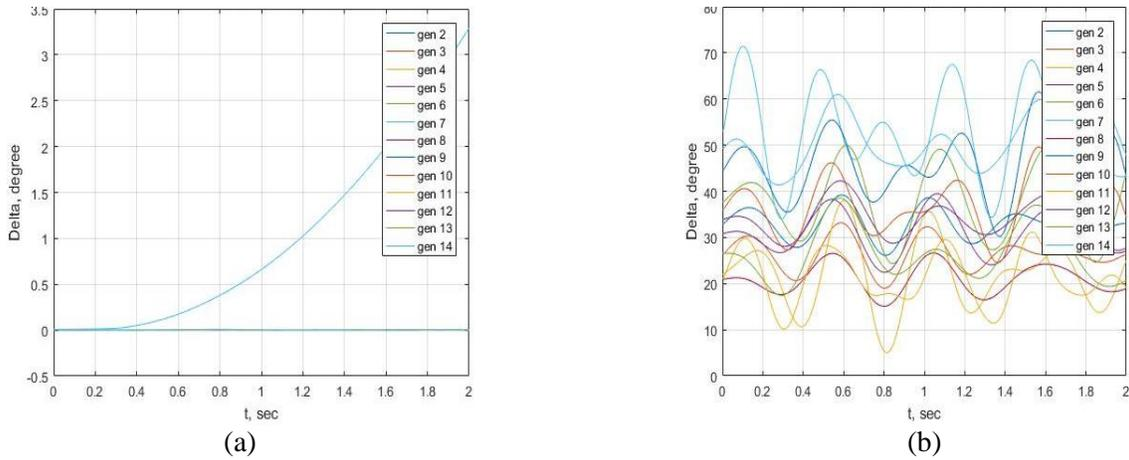
**Figure 10:** Swing curve of three-phase fault on bus 22, line [22-29] of the Nigerian 34-bus power network and cleared at 0.0132 s (a) without STATCOM (b) with STATCOM
