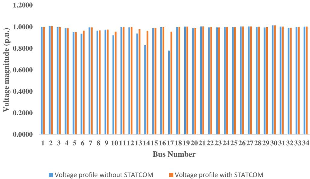
**Figure 3:** Voltage magnitudes of the Nigerian 34-bus power network
