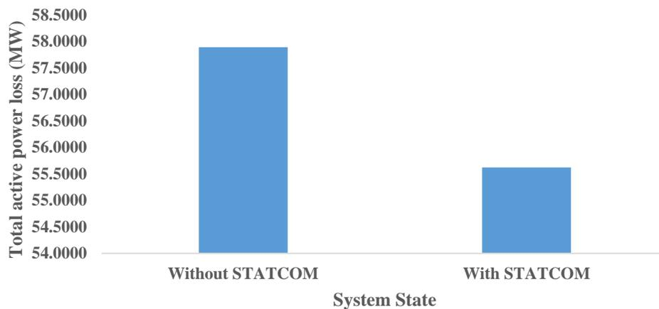
**Figure 4:** Total active power loss of the Nigerian 34-bus power network
