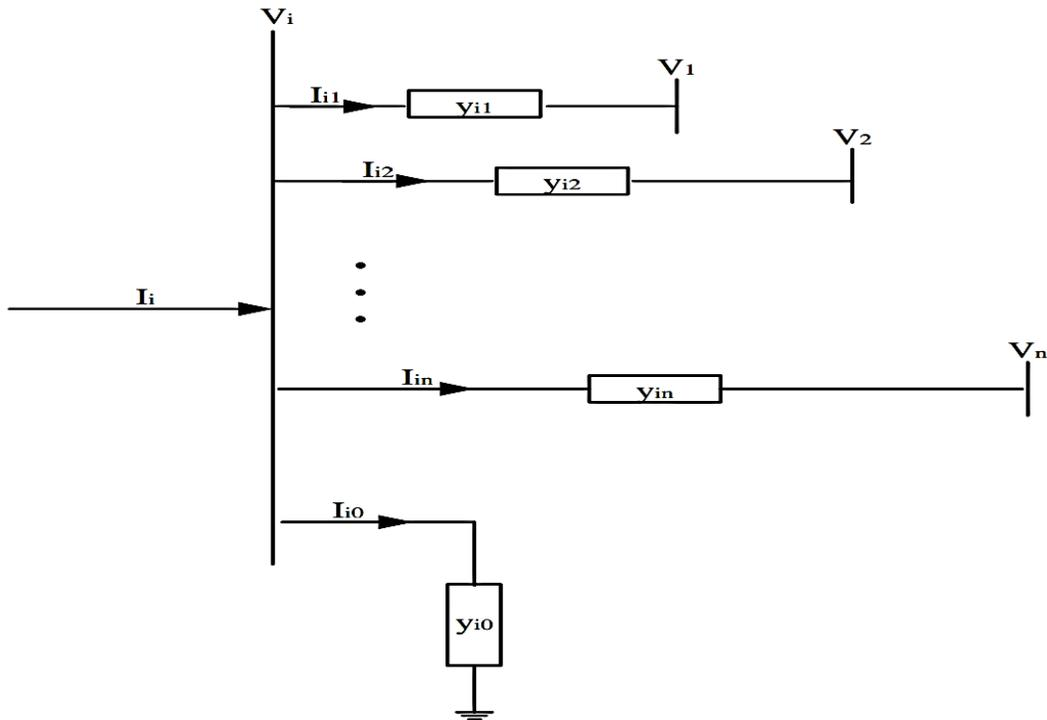
**Figure 1:** An n-bus structure of power system (Gupta, 2011; Hadi, 2008; Kothari and Nagrath, 2008)
