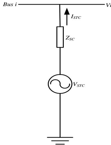
**Figure 2:** Thevenin's equivalent circuit of STATCOM (Jokojeje et al., 2015a; Jokojeje et al., 2015b)
