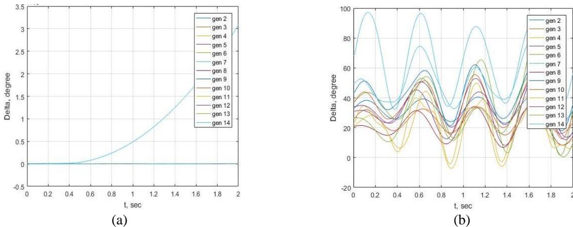
**Figure 7:** Swing curve of three-phase fault on bus 20, line [15-20] of the Nigerian 34-power network and cleared at 0.020 s (a) without STATCOM (b) with STATCOM
