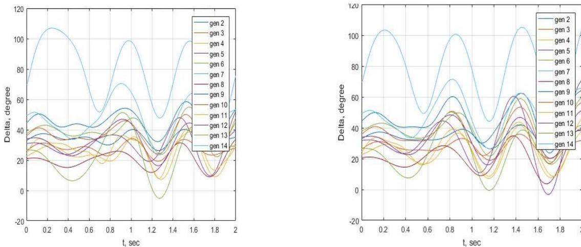
**Figure 9:** Swing curve of three-phase fault on bus 22, line [22-29] of the Nigerian 34-bus power network and cleared at 0.013 s (a) without STATCOM (b) with STATCOM
