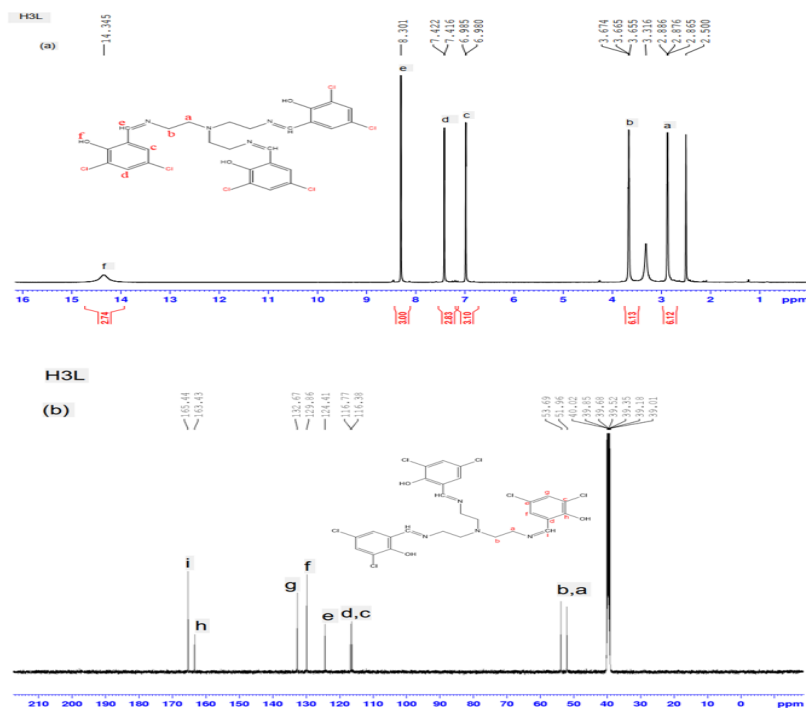
Figure 1: (a) 1 H NMR (500 MHz, DMSO- d 6 ) and (b) 13 C NMR (125 MHz, DMSO- d 6 ) spectra of the tripodal Schiff base ligand H 3 L synthesized from tris(2-aminoethyl)amine and 3,5-dichlorosalicylaldehyde. The resonance assignments are indicated using the lettering scheme shown in the inset molecular structures. Owing to the molecular symmetry, only one of the three chemically equivalent salicylidene arms is labelled.
