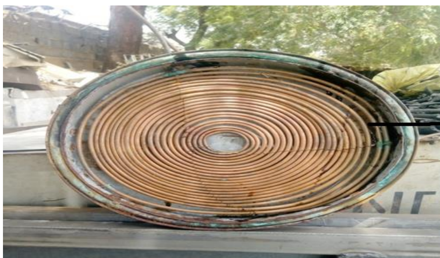
Figure 5: Spiral coil receiver- absorber with insulating cover
