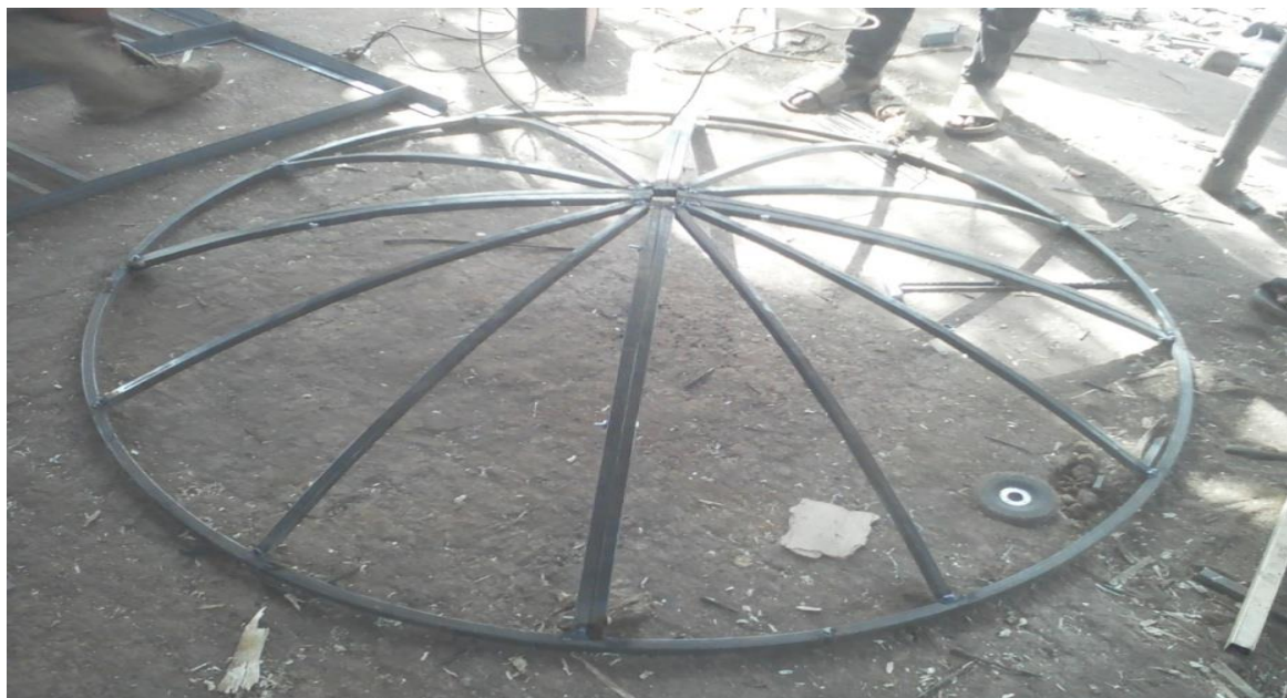
Figure 2: Assembled of trapezoidal petal-shaped reflector of parabolic dish concentrator
