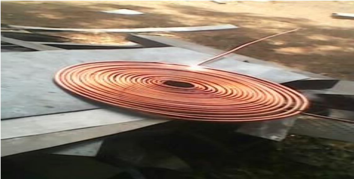
Figure 4: spiral coil receiver- absorber without insulating cover
