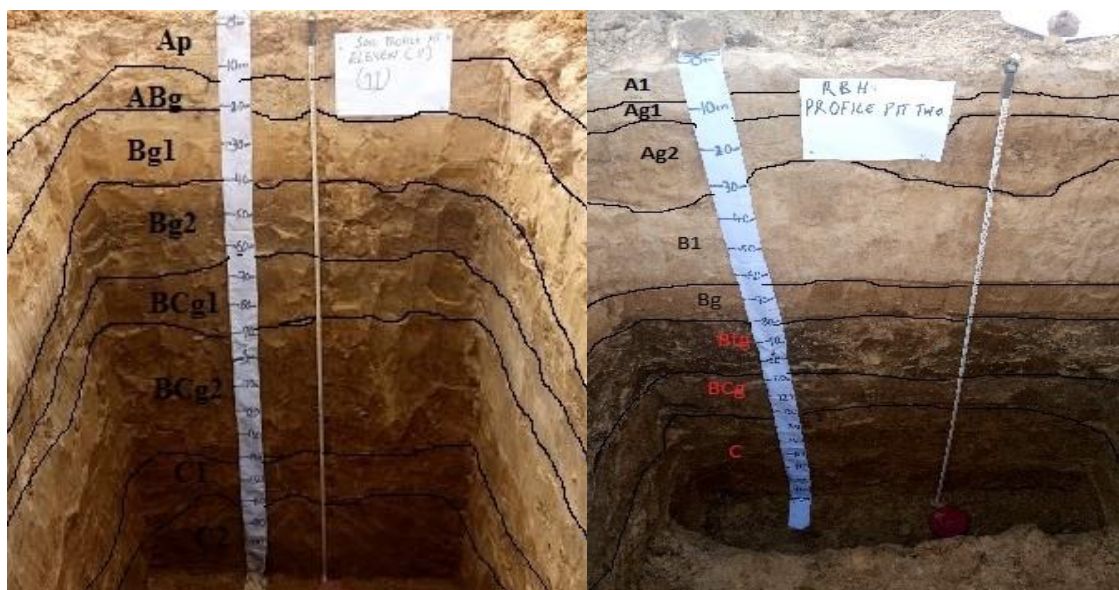
Plates 4 and 5: Profile Pits of Hauki 1 series (RBH2) Pedon P3 and P4 showing different horizon designations
