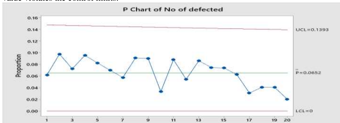
Figure 9: Control Chart for Friday production Number of groups = 20, Center = 0.0652, LCL = 0.00, UCL = 0.1393, StdDev = 1.667 Number beyond limits = 0, Number violating runs = 0. Figure 9 indicates that all the points in the chart are within the range of control limits. Hence, conclude that the proportion of number of defectives is under statistical quality control.
