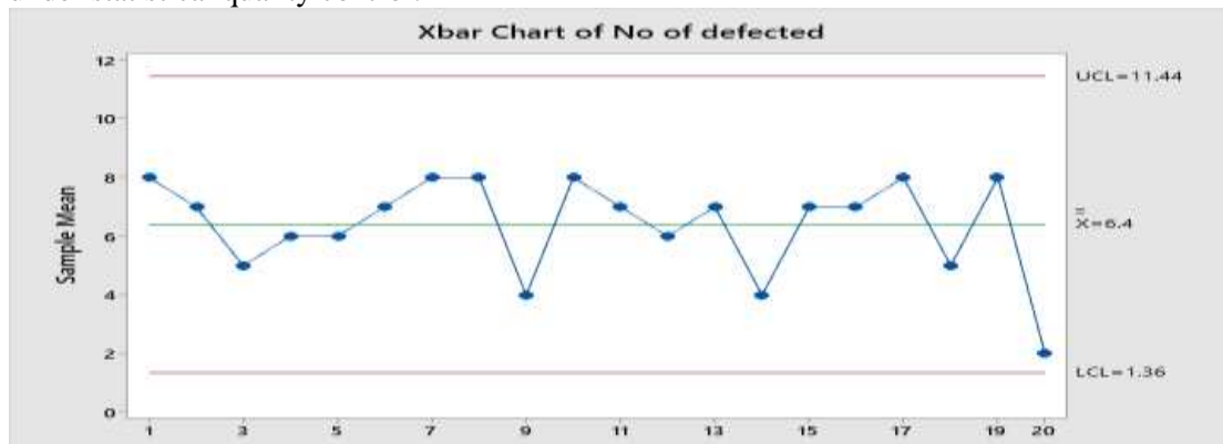
Figure 8: Show the X- bar chart for Thursday production Number of groups = 20, UCL = 11.44, Center = 6.40, LCL = 1.36, StdDev = 1.944 Number beyond limits = 0, Number violating runs = 0. Figure 8 further ascertain that Atlantis Bottle Water do conform to world Health organization standard. Hence, the water is adequately under control as no value violates the control limits.
